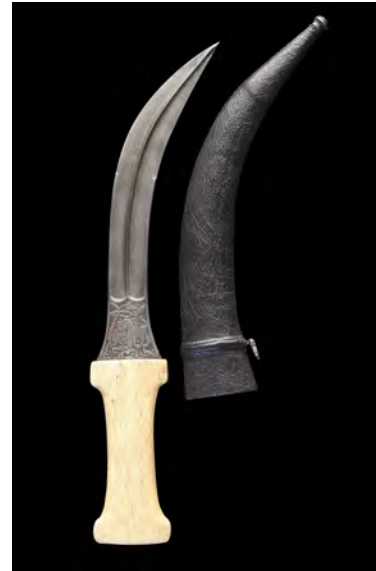
Fig. 24. A Persian khanjar with a patterned crucible steel blade.
